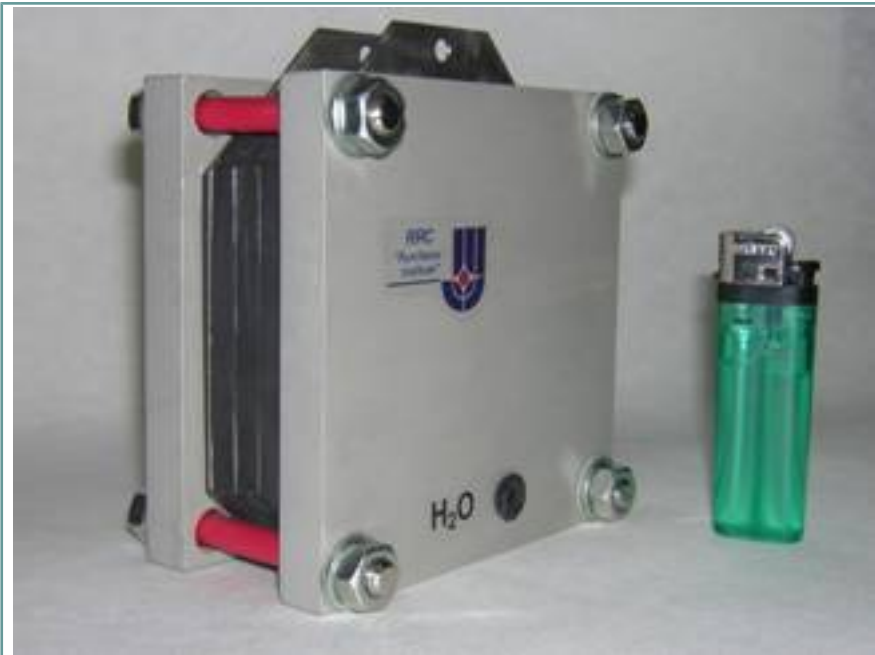
Fig. 1. A photo of PEM water electrolyser with productivity of 25 l/hour
