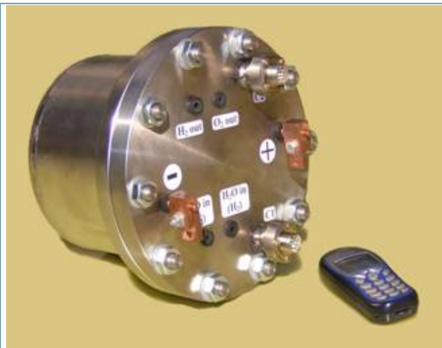
Fig. 2. A photo of PEM water electrolyser with productivity of 125 l/hour (operating pressure up to 30 bar)
