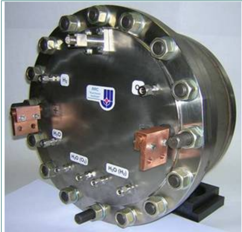
Fig. 3. A photo of PEM water electrolyser with productivity of 1,5 m 3 /hour, operating under pressure to 30 bar
